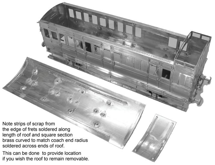
With the roof components fitted that should be all of the metal component construction completed.
