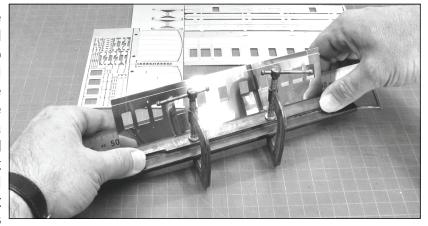
the bottom of the side with a flat file to give a crisp outside edge. Don't reinforce this fold before assembly of side and ends or you wont be able to tweak any slight adjustments into the bottom strip to make it completely flat.
