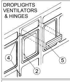
Fit the door ventilators (parts 5) centrally into the top panels (remember that the vents for the brake doors are marked parts B5). I tin the backs first and then holding them into place with a knife point and using plenty of flux sweat them into place using only a small amount of solder on the iron bit therefore requiring very little cleaning up.
