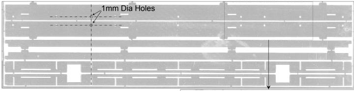
There are a couple of 1mm diameter holes for the footboard supports that I missed putting on the solebars. It is easier to mark and drill these before removing parts from the fret as the etched rebates (for the 0.9mm wire supports) on the back of the footboards can be projected up to determine the hole positions.
