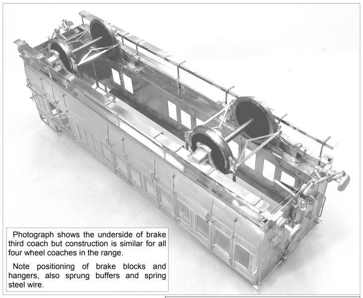
The buffers on the prototype coach 9. were of an unusual type. They had a short and distinctly shaped body with a long buffer shaft and a thick wooden faced head. Because of this they do not lend themselves so easily to produce sprung buffers by my usual method so I have provided alternative solid buffers that you may wish to use.
